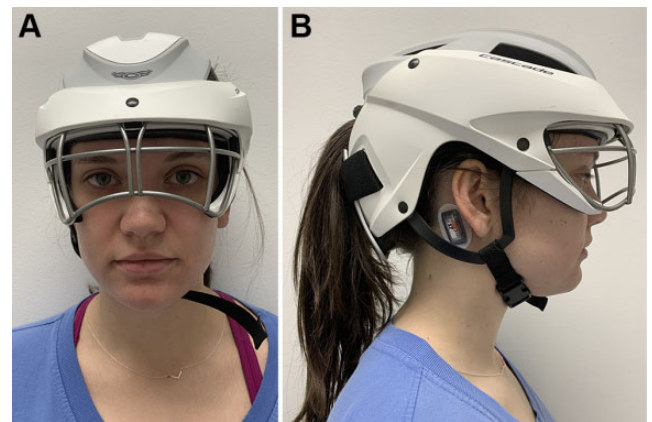
Figure 1. (A) Front and (B) lateral views of lacrosse headgear and wearable sensors affixed behind the ear.
